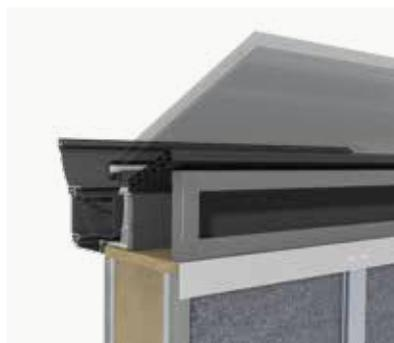
A top tray runs along the top of the hup! walls underneath the eaves beam. The clips are secured into place by fixing through the top tray. Raked frames must be used on lean-to roofs as the walls cannot be raked and meet a glass panel/ starter bar
