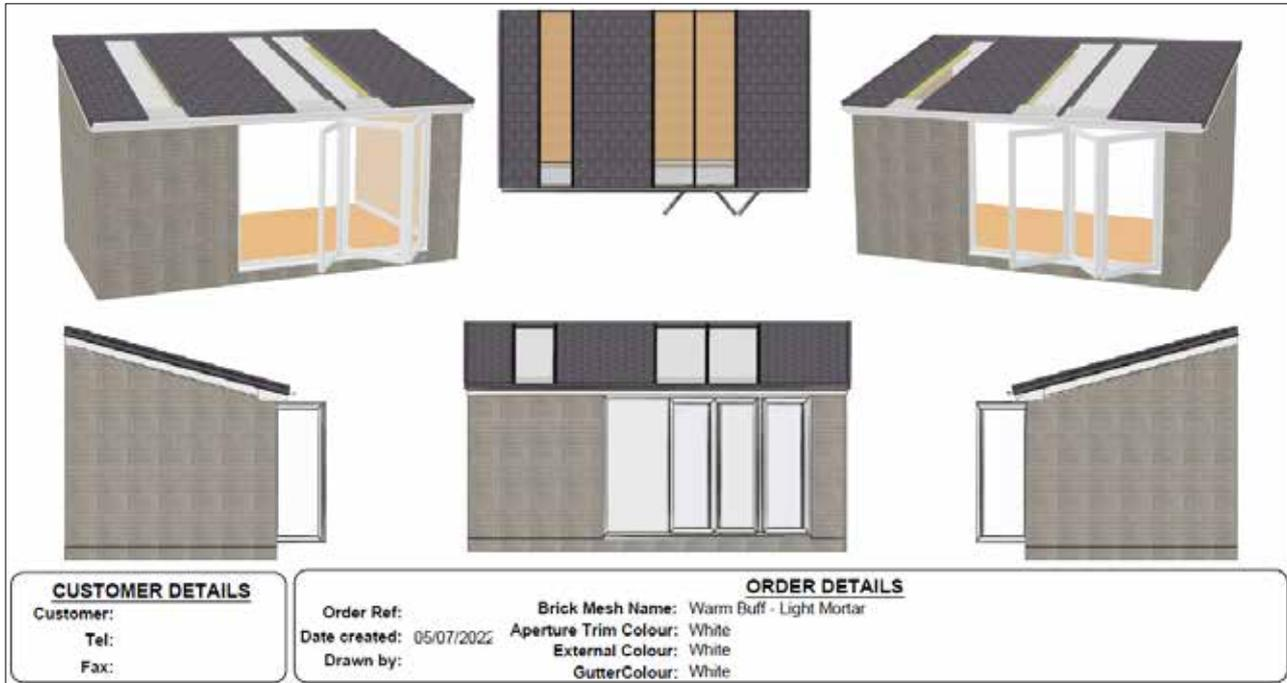
This shows a 3D representation of the hup! from all sides. A single glazed roof panel lights the utility room, and bi-fold doors and a double glass roof panel provide plenty of natural light into the lounge. Both boundary walls are solid with no windows. White gutters and roof trims have been chosen and the walls are shown with the hup! Brick Mesh in Warm Buff with Light Mortar.
