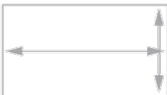
Measure lengths of base. Acceptable deviation is: +/-30mm overall on width and +/-15mm on projection.
