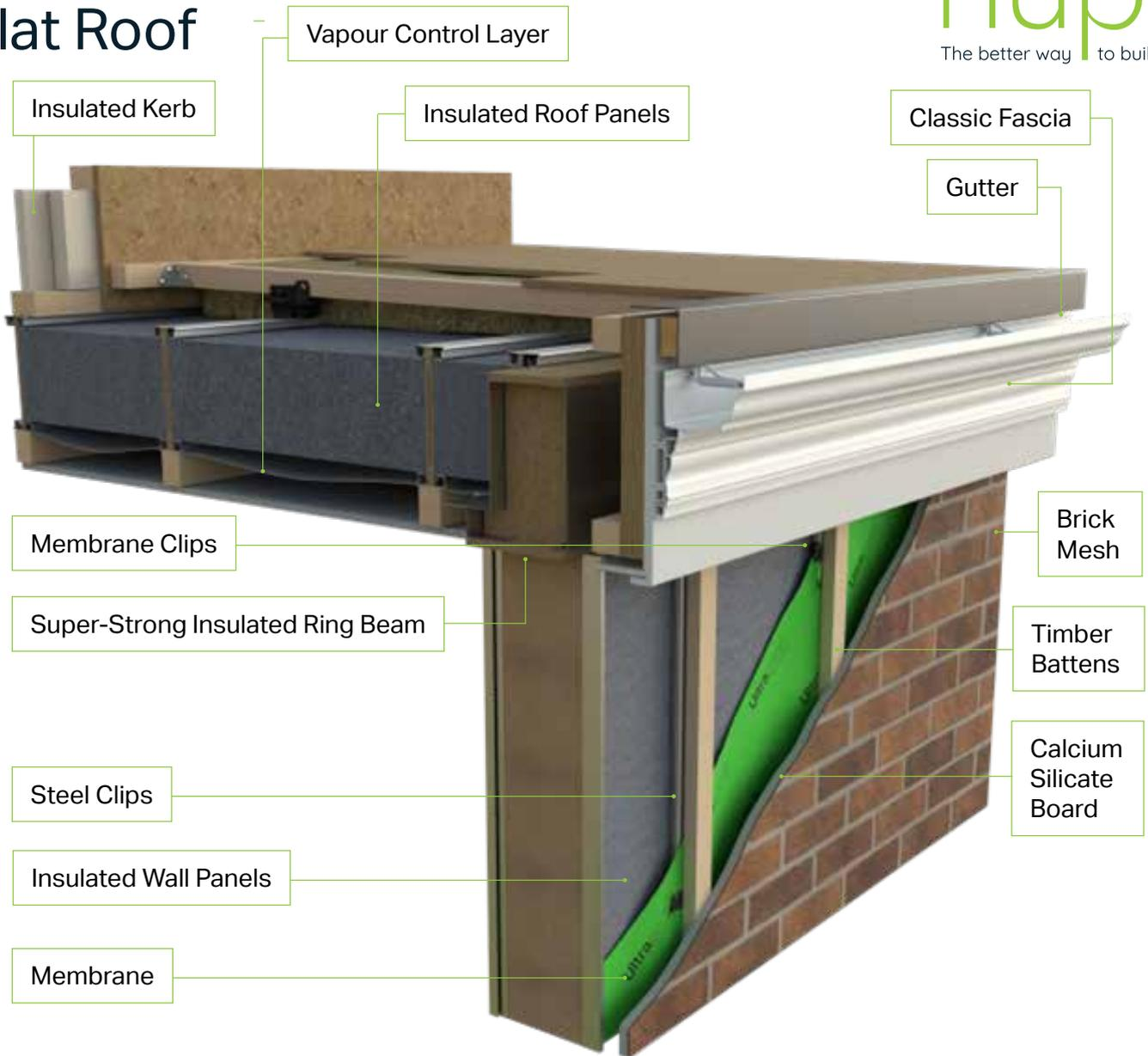
The hup! Flat Roof system is available in rectangular shapes up to 4m projection and 7m wide. With all structural calculations taken care of in one easy order the hup! Flat Roof can accommodate 0, 1 or 2 apertures and supplied with lanterns or flat skylights as required.
