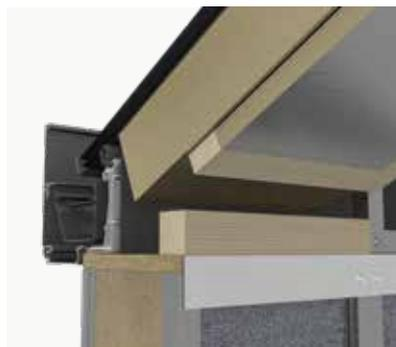
A top tray runs along the top of the hup! walls underneath the eaves beam. The clips are secured into place by fixing through the top tray. Raked frames must be used on lean-to roofs as the walls cannot be raked and meet the panels/ starter bar.
