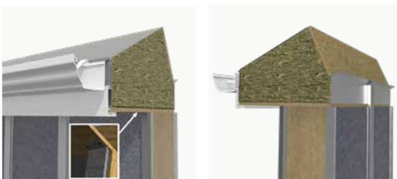
The clips run up the back of the internal side of the beam and are screwed into the steel beam section.
